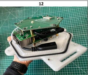
Plug in the micro-USB to USB-C right angled connector and pass through the device as shown.
