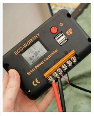
2. Connect the solar panel to the solar charge controller by the AWG10 wire. Ensure you connect positive to positive and negative to negative. Left two terminals in the picture here.
