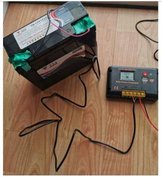
3. Connect the Battery to the solar charge controller (middle two terminals). You can use the AWG10 for this or I've often just used the wires that came with the panel/solar charge controller set. Again, ensure you connect positive to positive and negative to negative. Note: the solar panel isn't attached here, but if for your field deployments make sure that it is.
