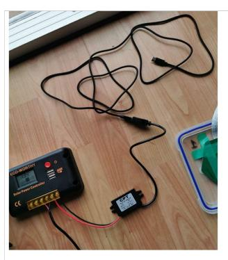
5. Attach the 12V to 5V step-down to the power out terminus on the Solar Charge Controller. Ensure the terminals match up and that the 12V side is attached to the solar charge controller. Right two terminals here. Note: Depending on the type of step-down converter you have you may need a USBC adaptor.
